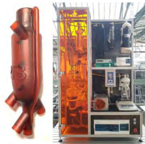
Figure 1: Continuous Energetic Liquid Agitation System (ConElia). Left: Mixing flow cell. Right: The completed device with mixing, pumping and monitoring parts.
